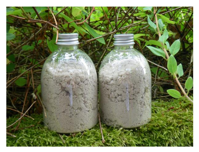
**Figure 7.3** Phosphorus recovered from wastewaters in the form of struvite produced from a Huber SE precipitation reactor. Photograph courtesy of The Sustainable Sanitation Alliance (SuSanA).
